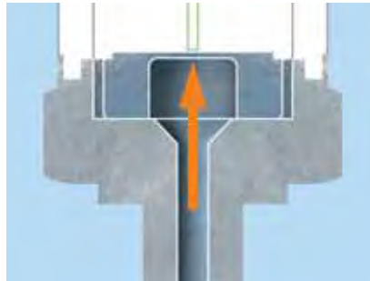
The welded stainless steel measuring cell – for diverse applications in gases and liquids up to 400 bar: e.g. hydraulics, gas, water, brake liquid or cryogenics (freons).
