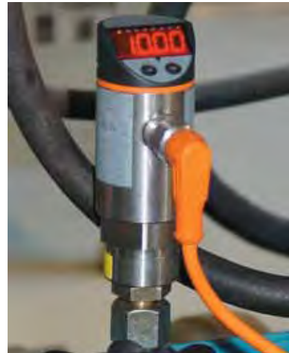
The display: The 4-digit, alphanumeric 10-segment display shows the system pressure at a glance.
