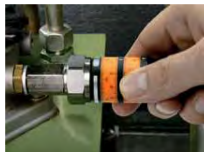
The easy turn operating concept: There is no easier way. Set and reset point adjustment with only two turns.
