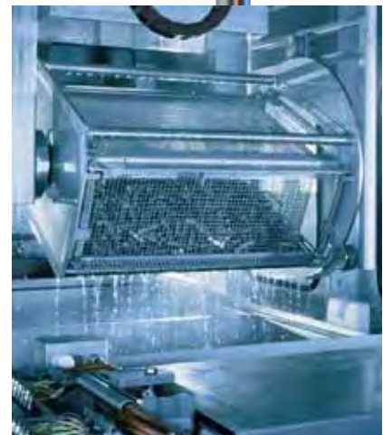
In industrial part washer applications the efector gwr reliably detects the level of aqueous cleaning agents at medium temperatures up to 80 °C.
